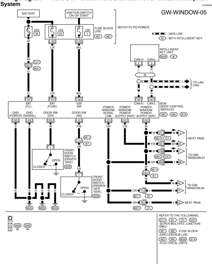
Wiring Diagram — WINDOW —/With Front and Rear Power Window Anti-pinch
