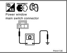
4. Check continuity between front power window switch (passenger side) connector D36 terminal 11 and ground.
